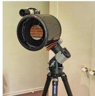
Fig. 2. The RH-200 and a closer view of the RST-135 in EQ mode. Note that there is no counterweight!
