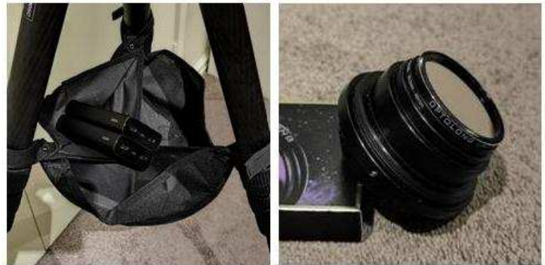
Fig. 5. Two compact Xiaomi power banks sitting in the stone bag attached to the tripod legs, and the Optolong 2" filter screwed into the Officina Stellare camera adapter.
